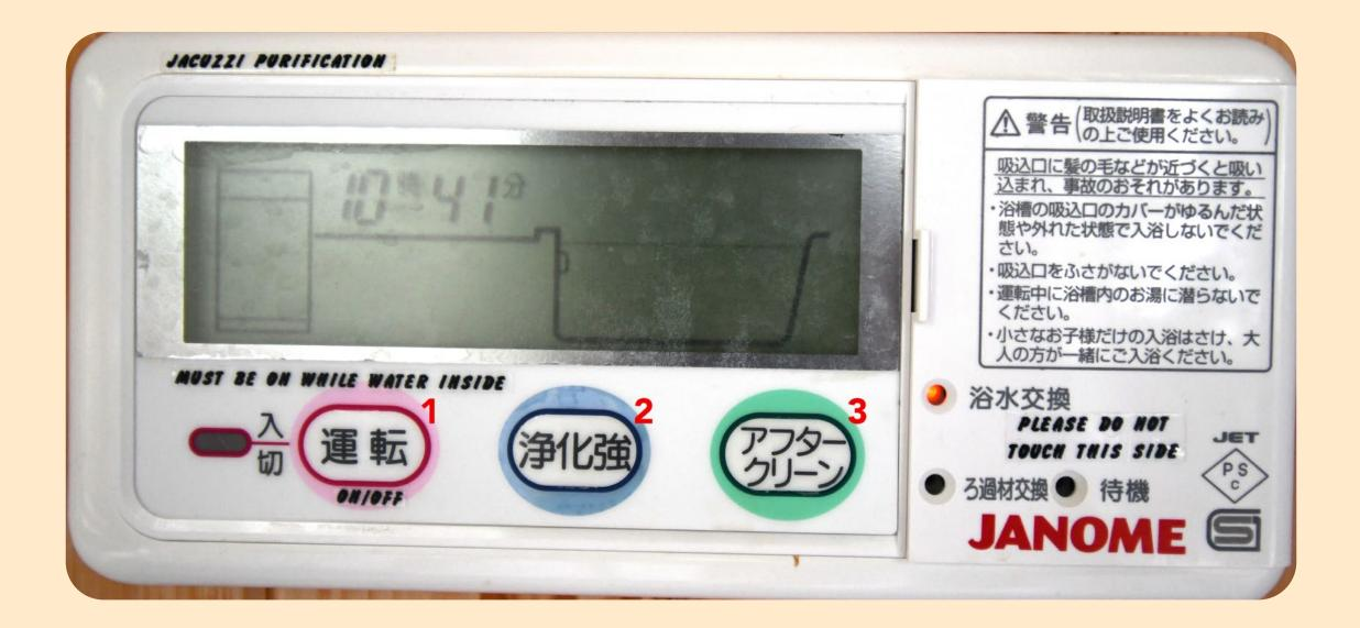
Once you have finished bathing, press BUTTON 1 to turn on the cleaning system, then press BUTTON 2 to start the clean.
